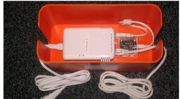
This seismometer plugs into your home router. The lid is removed to reveal the hardware
